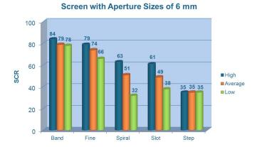
WEF, in co-operation with ASCE, conducted a study<sup>1</sup> of the screenings volume relative to flow collected at 39 US wastewater treatment plants. Results proved that plant screenings are so unique, they differ by a factor of 70. Even conservative sizing methods used by most engineers cannot properly account for fluctuations in screenings of this magnitude when calculations are based on peak flow and opening size alone.
